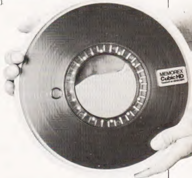
Good, old-fashioned magnetic tape. 2400 feet at 6250 BPI equals an awful lot of information.
